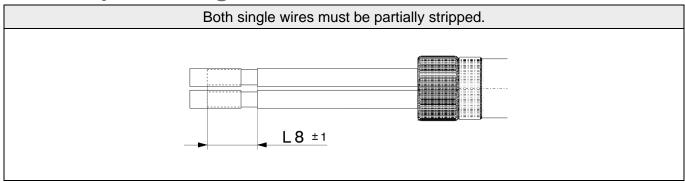
When stripping the wires, the conductor may not be damaged.
