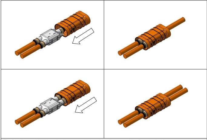
The Distributor shield housing is symmetrical and can be assembled from both sides. During assembly, locking latches in the shield are deflected and lock audible.
