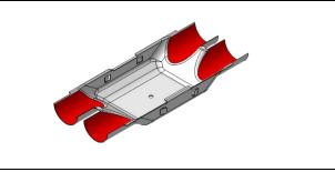
Do not damage the following parts during the pressing process.
