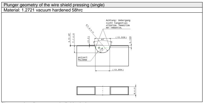
Plunger and anvil are geometrically identical.
