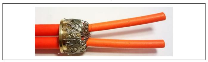
Do not cause any mechanical damages on the single conductors during the manufacturing process. If necessary, the twisted shield netting can be dissolved (brushed off).
