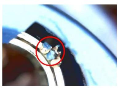
Pictures: HCT4 female contact holder, coding C with plastic chip
