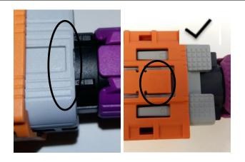
The CPA (grey part) is closed when the closed lock and arrows are visible.
