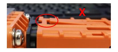
If the connector is not at the final position, the locking hook stays outside. Movement of the CPA (grey part) is not possible.
