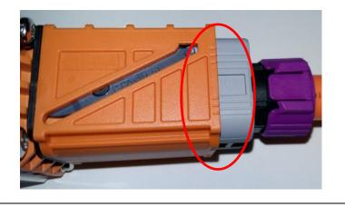
Pulling back by holding at marked area on both sides simultaneously.
