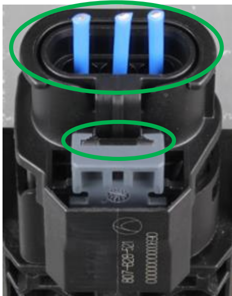
I.O. Gesteckt housing in end-lock position
