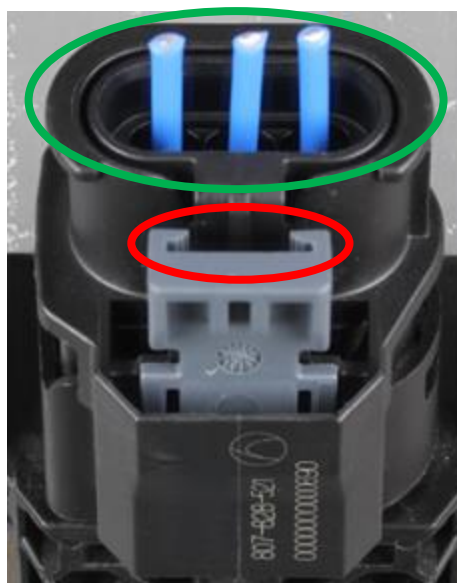
CPA in Vorraststellung CPA in pre-lock position
