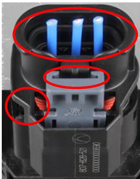
Kontaktträger + Schutzkragen + CPA in Vorraststellung female housing + shroud + CPA in pre-lock position
