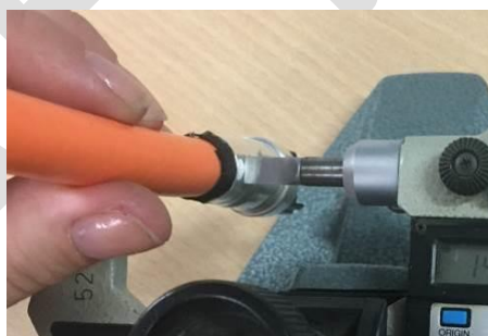
Figure 51: schematic representation of the measurement of the pressing height
