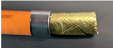
Figure 24: Assemble the stress relief
