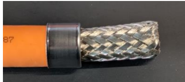
Figure 25: remove the foil
