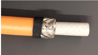
Figure 28: Fold over and fix the shielding
