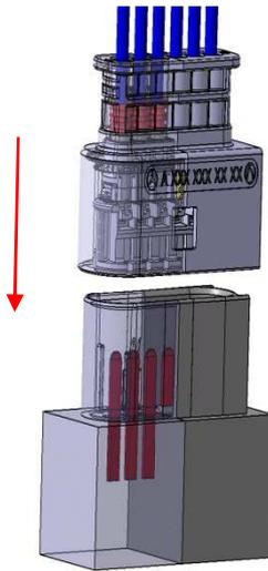
The plug-in connection is completed by inserting vertically in a suitable unit connection or pin housing until the clip is correctly engaged. Engaging of connector housing in counterpart is ensured by clicking. After a correct connection the CPA, if available, can be engaged with is also ensured by clicking.
