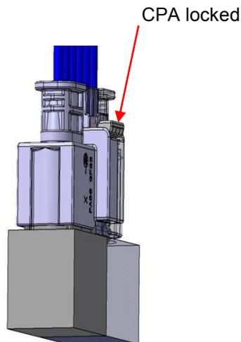
Ideally the connector is inserted vertically in the suitable unit connection or pin housing by pushing directly on the CPA. In this case the connector and the CPA are engaged in one step.
