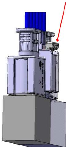
The SealStar 2.8 Housing is held positively in the unit connector. To disconnect it, firstly the CPA, if available, has to be pulled in the pre-engaged position. After this the SealStar 2.8 Housing can be disconnected by deactivating the clip and pulling in the direction of the wire.
