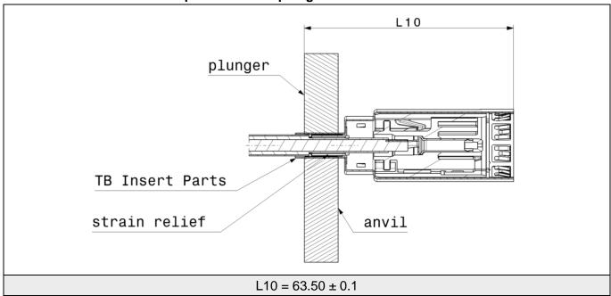
The chamber on both anvil and plunger must face towards the shield-sleeve.
