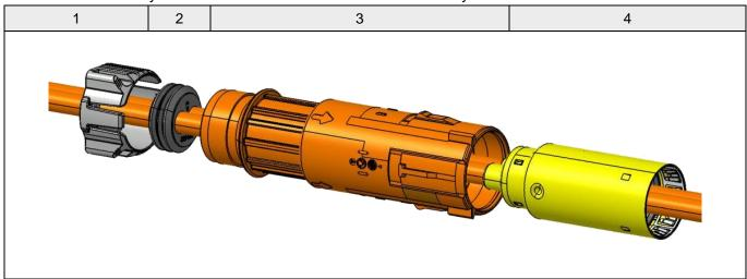
Note: The (TB) male Housing unit (3) and shielding sleeve (4) may as well be assembled onto the cable after crimping of HCT4-male terminals.
