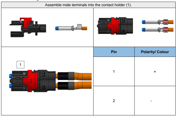
While assembling the HCT4 male terminals, the terminal will audibly engage oonce the end position is reached. The male terminals must be crimped. When two wires with the same colour are used, the pinning must be confirmed via electrical testing.
