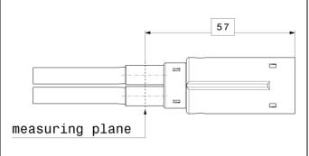
To check the dimension "d", the height needs to be measured acc. to the drawing.
