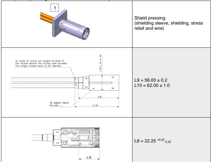
The dimension L9 and L10 are just for information. The dimensions are given through the dimensions L1, L4 and the EVS-100068.
