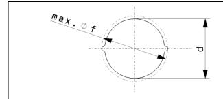
The plunger and anvil are pressed together to 0.2 mm clearance. Due to this, the dimension "d" will be given. See table of each cross section.
