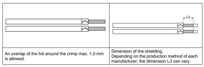
After cutting the shielding, there are no wire residues or parts of the shielding allowed on the cable. This must be ensured with some actions like the following:
