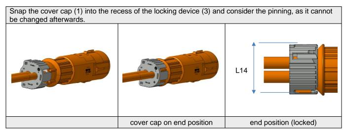
Do not damage the cover cap (1) or the seal (2) during assembly. If the cover cap is in end position, the locking hooks must be straight on both sides and are not allowed to be deflected. They must be within L14 = max 25.0 mm.
