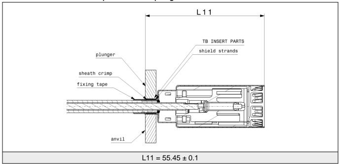
The chamber on both anvil and plunger must face towards the shield-sleeve.
