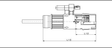
During the assembling process, there are no damages allowed on the shield sleeve, the contact carrier, or the wire. There is no pull on the wire necessary. Especially do not pull out the cable sheath out of the stress relief.
