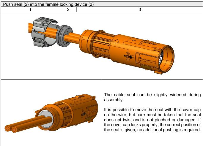
The seal is lubricated, no additional lubricants are permitted.
