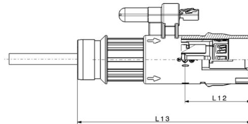
During the assembling process, there are no damages allowed on the shield sleeve, the contact carrier, or the wire. There is no pull on the wire necessary. Especially do not pull out the cable sheath out of the stress relief.
