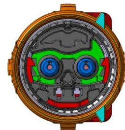
Since there is literally no geometry it is recommended to measure circumferentially on the plastic housing.
