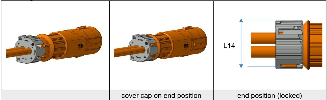
Do not damage the cover cap (1) or the seal (2) during assembly. If the cover cap is in end position, the locking hooks must be straight on both sides and are not allowed to be deflected. They must be within  $L14 = \max 25.0 \text{ mm}$ .
