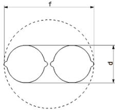
The plunger and anvil are pressed together until block. Due to this, the dimension “d” will be given. See table of each cross section.
