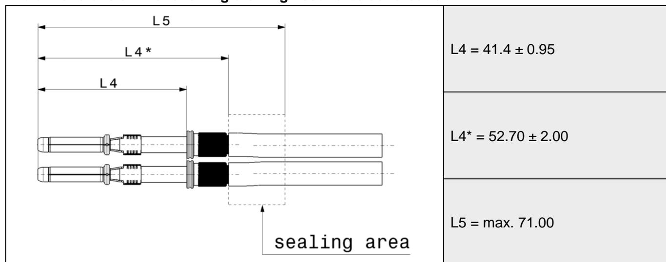
The dimension L5 and L6 are for information only. The dimensions are given through the dimensions L1, L4 and the EVS-100068.
