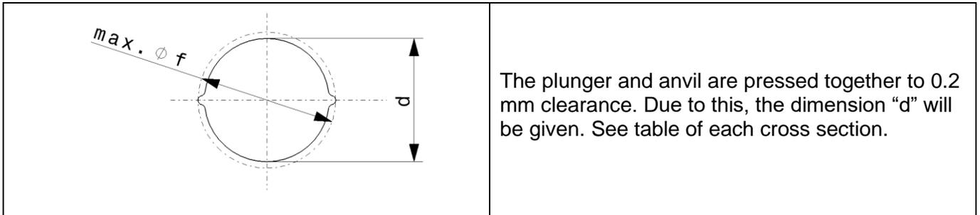
The plunger and anvil are pressed together to 0.2 mm clearance. Due to this, the dimension “d” will be given. See table of each cross section.
