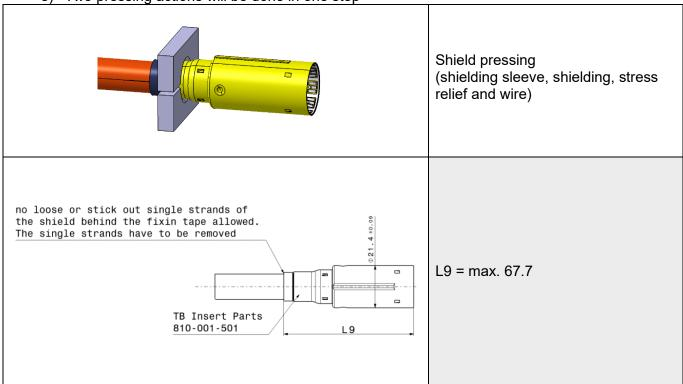
The dimension L9 is for information only. The dimensions are given through the dimensions L1, L4 and L8 and the EVS-100113.
