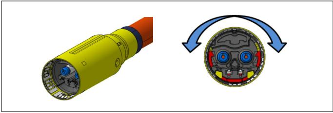
A <u>maximum rotation of up to  $\pm$  180°</u> is possible and cannot be exceeded. This twisting results in an overturning of the single wires, which leads to a reduction in length between the contact carrier and the strain relief. The movability must be ensured at least on one side (by the contact carrier or cable) to enable the length reduction.
