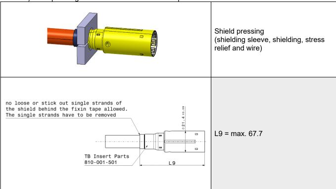
The dimension L9 is for information only. The dimensions are given through the dimensions L1, L4, L8 and the EVS-100113.
