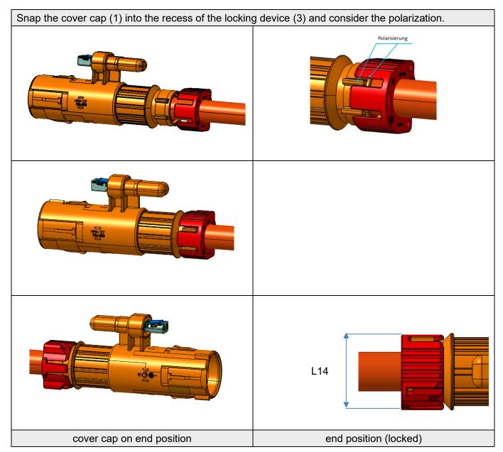
Do not damage the cover cap (1) or the seal (2) during assembly. If the cover cap is in end position, the latching hooks must fit directly on the female locking device unit on both sides. They are not allowed to stay in a deflected position. They must be within the dimension L14 = max. 25 mm. If the 90° angled cap is used, the processing steps of the cover cap (1) is omitted.
