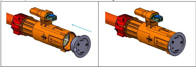
Insert the transport protection cap until both locking elements snap over the front collar of the connector housing. It is possible to turn the transport protection cap 360° during and after the assembling.
