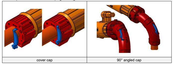
Ensure that the coding/ color of the coding clip matches the coding/ color of the built-in contact carrier. Therefor bars are attached to the coding clip according to a binary code which can be checked mechanically. The design of the bars can be found in the individual drawing of the coding clip.
