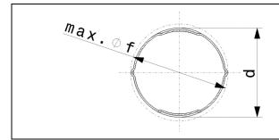
The plunger and anvil are pressed together until block. Due to this, the dimension "d" will be given. Therefore, see table of each cross section.
