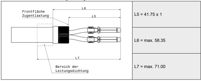
The dimension L5 and L6 are for information only. The dimensions are given through the dimensions L1, L4 and the EVS-100068.
