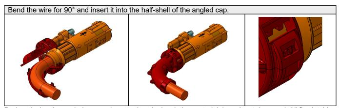
During closing the angled cap, make sure the wire insulation material doesn't get damaged. All five latching hooks must be locked. Once the angled cap is closed, it is not possible to change the angle.
