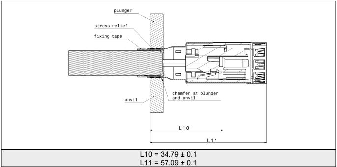
If the position point is on the base area of the contact holder, the relevant dimension for the anvil and plunger is L10. If the front area of the shielding sleeve is the position point, then L11 needs to be used.
