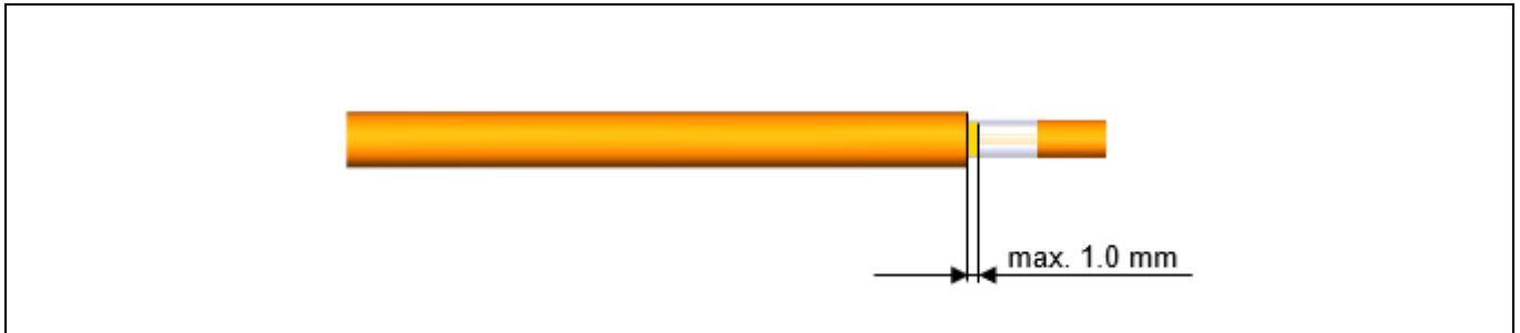
Figure 4.9: Representation 6.0 mm 2 SCC overhang shielding foil (4.4 Remove shielding foil (if present), trim shielding braid, and assembly the stress relief and X-Ring)
