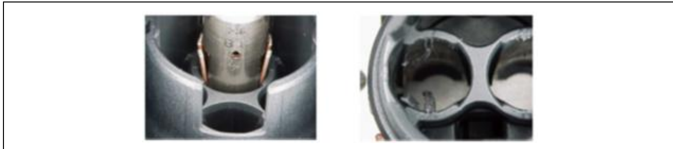
Figure 3.26: Representation 4.0 mm 2 SCC plastic burr on contact carrier (3.7 Inserting HCT4 female terminals into contact carrier)
