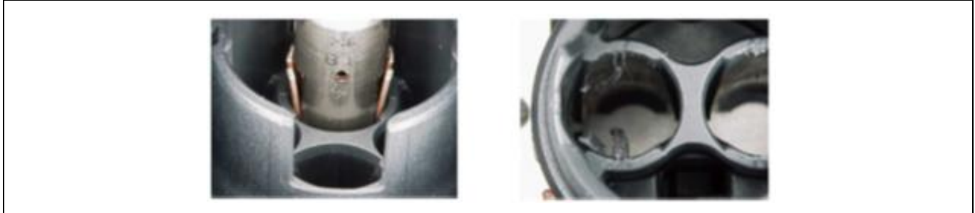
Figure 4.17: Representation 6.0 mm 2 SCC plastic burr on contact carrier (4.6 Inserting HCT4 female terminals into contact carrier)
