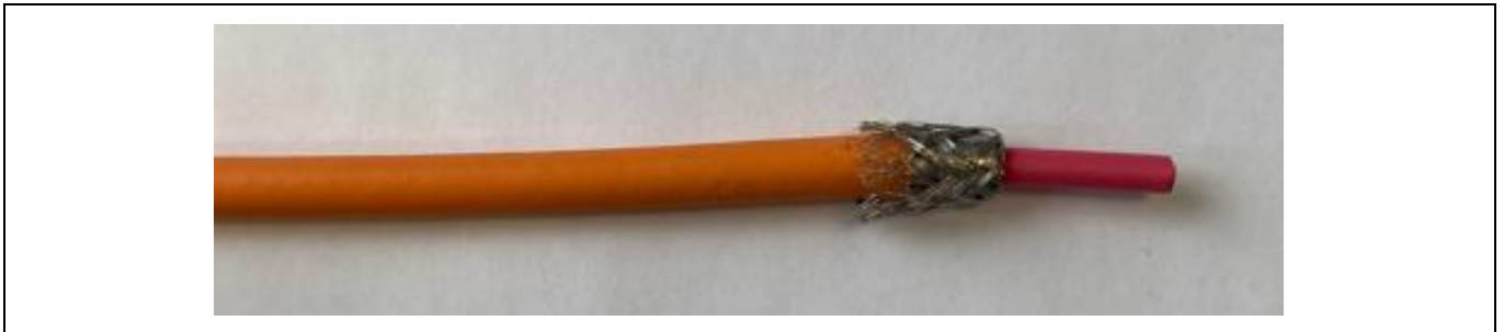
Figure 3.14: Representation 4.0 mm 2 SCC preserved shielding braid (3.5 Fold over the shielding braid and secure the shielding braid)
