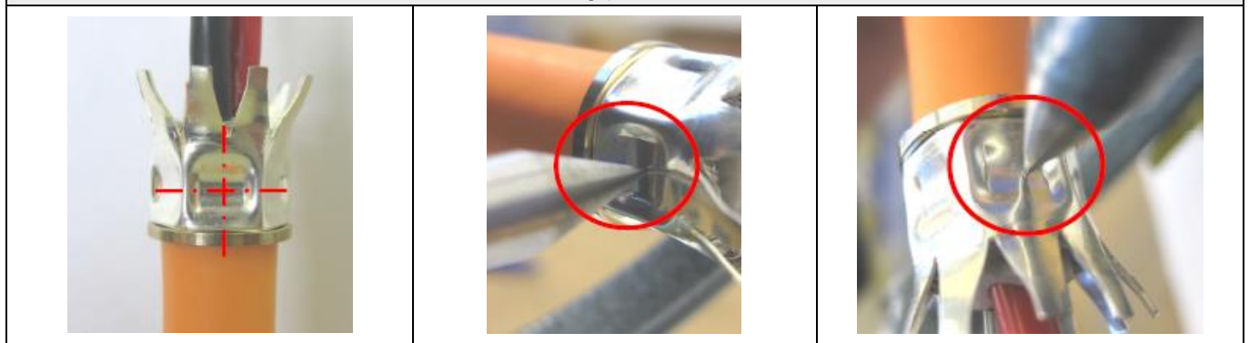
Position measuring points: center to center
